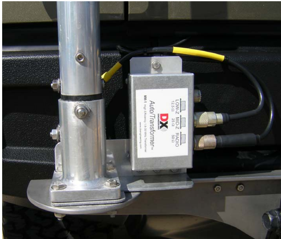
Figure1: MM-1 Installed on Vehicle
