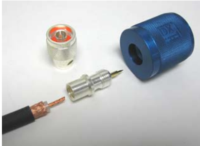
Coaxial cable properly prepped
