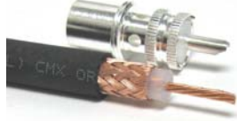
Properly prepare coaxial cable
