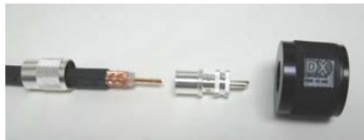
Insert coaxial cable into PL-259
